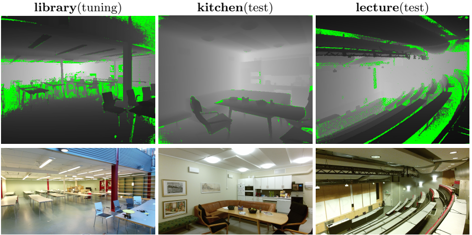
Fig. 3. Unwrapping ground truth for the three datasets. Top row: ground truth depth maps. Green pixels are suppressed, and not used in the evaluation. Bottom row: corresponding images from the RGB camera.
