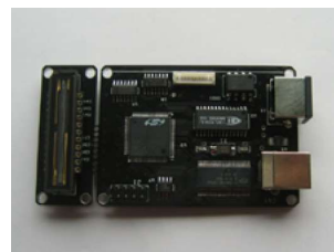
Mightex 3648-pixel line camera
