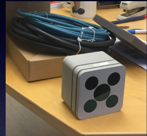
Fotonic (Veoneer) Prototype ToF camera
